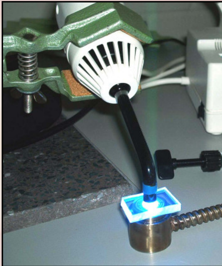
DEA experimental set-up investigation of primary-curing
