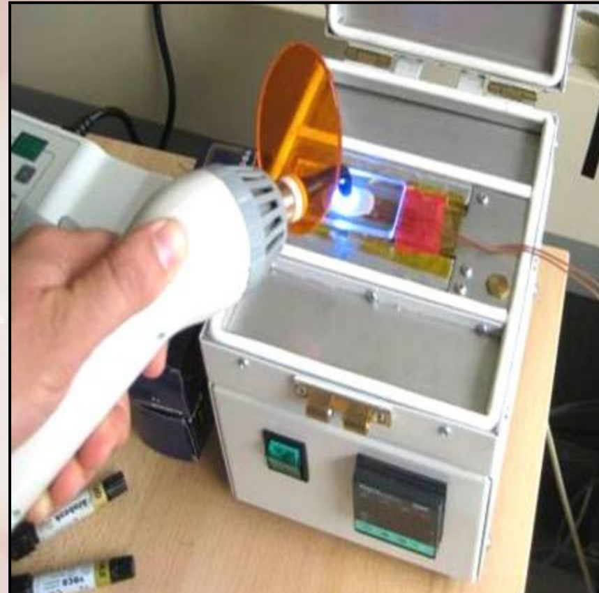
DEA experimental set-up investigation of post curing 36 °C
