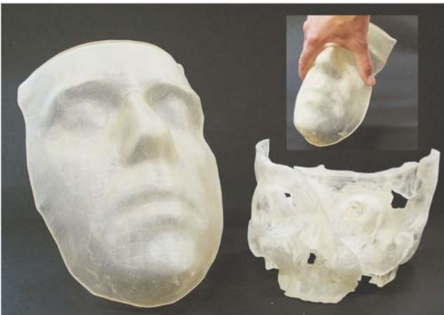
Notes: Soft tissue model, realized using FlexSL SM-25 (left picture & insert) and an skull model for intra-OR use (FlexSL SM-1500 material, lower right picture)
