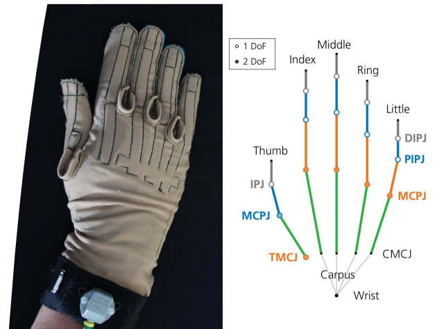
Figure 1: Dataglove used for recording joint angles (left, CyberGlove Systems LLC right hand CyberGlove) and schematic kinematic chain of a human hand (right). The abbreviations used for joints in the kinematic chain stand for (proximal, distal) interphalangeal joints (PIPJ, DIPJ, IPJ), metacarpophalangeal joint (MCPJ), carpometacarpal joint (CMCJ) and trapeziometacarpal joint (TMCJ). Filled circles represent joints with two degrees of freedom (DoF) in that joint, unfilled circles represent joints with one DoF.
